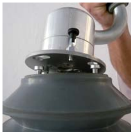
Quick-change coupling for exchanging the suction feet for different tasks during ongoing operation
